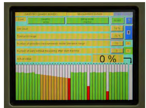
savePro® Powder Monitor. Measured data are visualized on touch screen.
